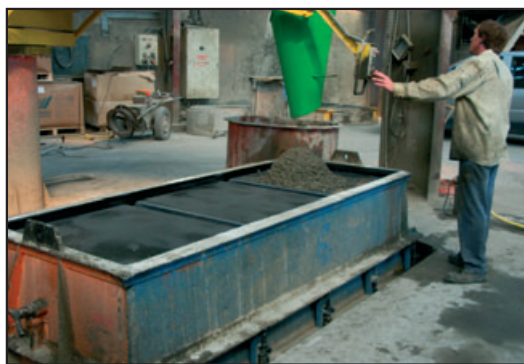
A 4 000 litre mould in a pit filled with water
