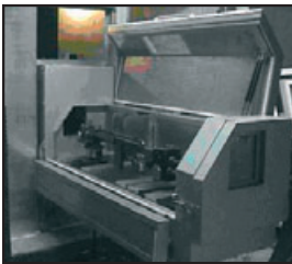
Enclosure with both upper main panel and with front panel open. (in order to adjust the holding)
