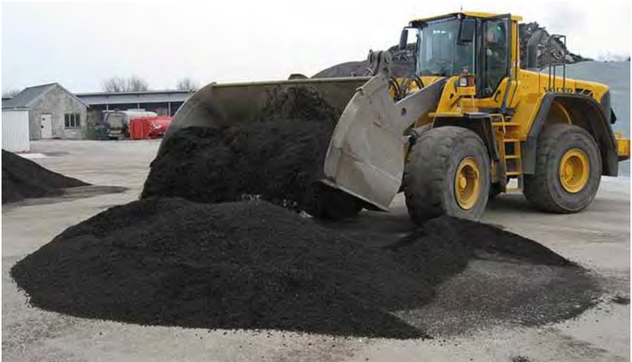
Asphalt produced from the recycled material has been proven suitable for most road surfacing uses
