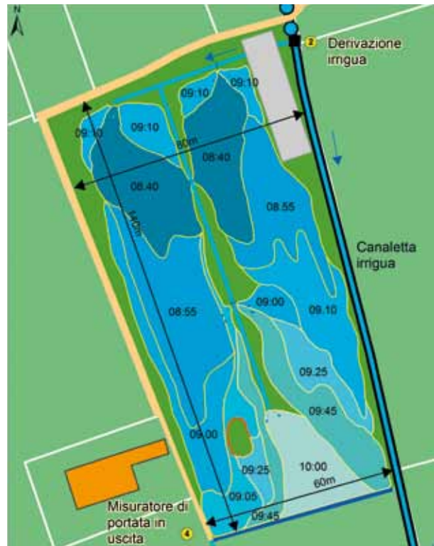
The test field and the progressive water distribution during the initial phases of water provision at the Busta site
