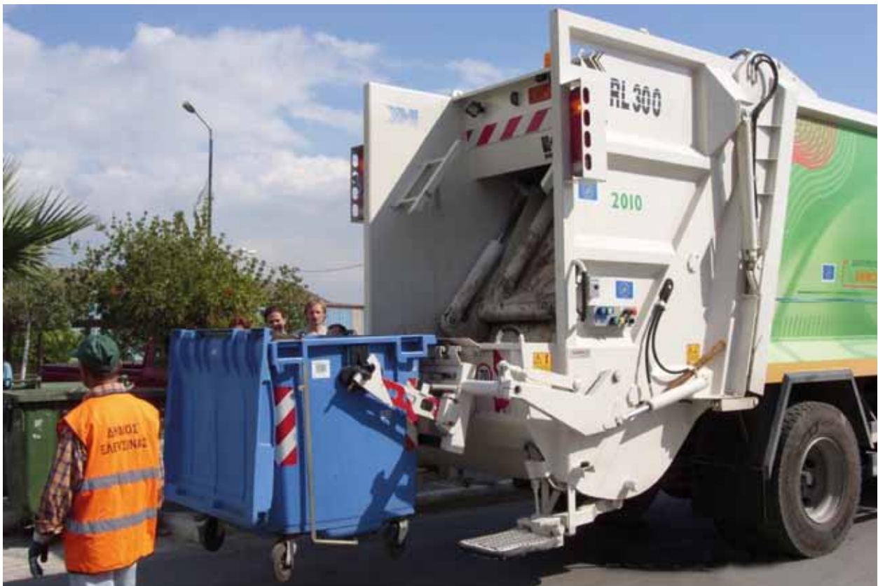
Refuse collection lorry with weighing equipment
