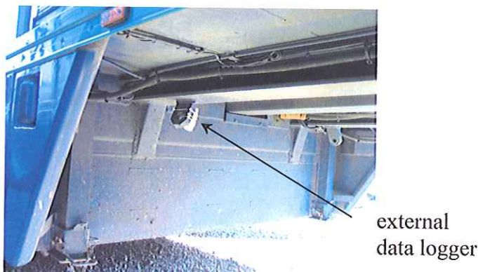
Picture III.3: Example of a data logger, installed under a semi-trailer for recording external temperatures/humidity
