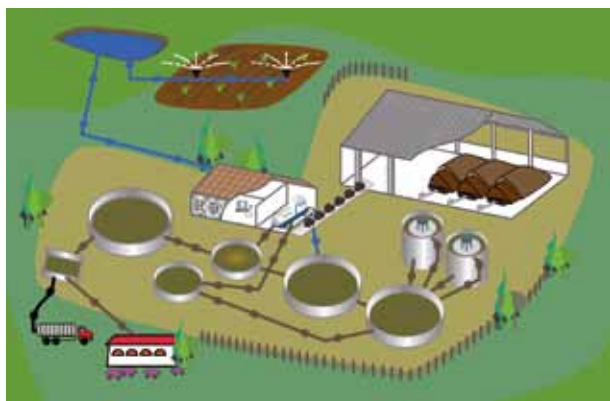
Schema of the treatment plant in Peñarroya de Tastavins, which treated 100 000 m 3 of slurry
